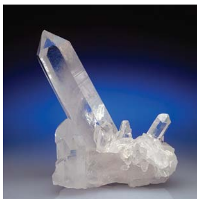
FIGURE 1-3 Quartz crystal Quartz (silicon dioxide) is the silicon analog of carbon dioxide. Whereas carbon dioxide is gaseous, silicon dioxide is a solid.
